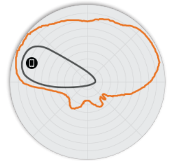
Figure 5. R720 5GHz Elevation Antenna Patterns
