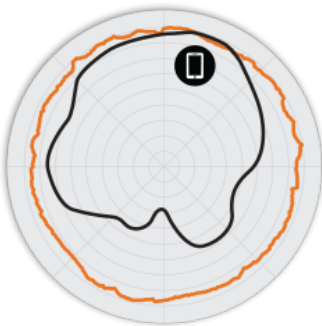
Figure 2. R720 2.4GHz Azimuth Antenna Patterns
